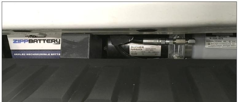
Standard operating procedure recommends starting the vehicle prior to running the pump to use the door or lift. IF the engine is not running the new system will no longer run off the vehicle's starting battery as it now pulls its power from the emergency backup battery when the engine is not running. Obviously, this benefits the starting battery by not draining it down if the user fails to start the vehicle prior to using the door or lift systems.
